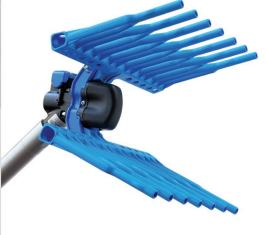
Classic style air powered harvester. A shortened piston stroke increases the beats per minute to 1800 and reduces the air usage from 200 to 150 litres per minute.
