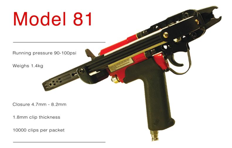
The SIMES MODEL 81 PNEUMATIC FASTENER is used to apply the Simes RT-23 CLIP when fastening during fencing, greenhouse and cage construction or repair. The pneumatic plier offers quick and easy application for large jobs.
